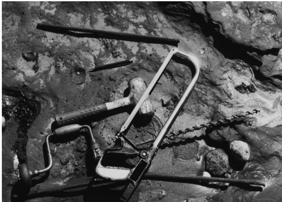
Figure 11. Some tools for marking a wave-cut platform. The carpenter's auger was used here to bore a hole in the glacially-compacted, peaty soil of the Whidbey Formation. The pencil points to the top of a piece of “rebar” (cut with a hacksaw), which has been driven flush with the wave platform surface. If erosion begins to expose the reference pin, you can simply pound it deeper.
