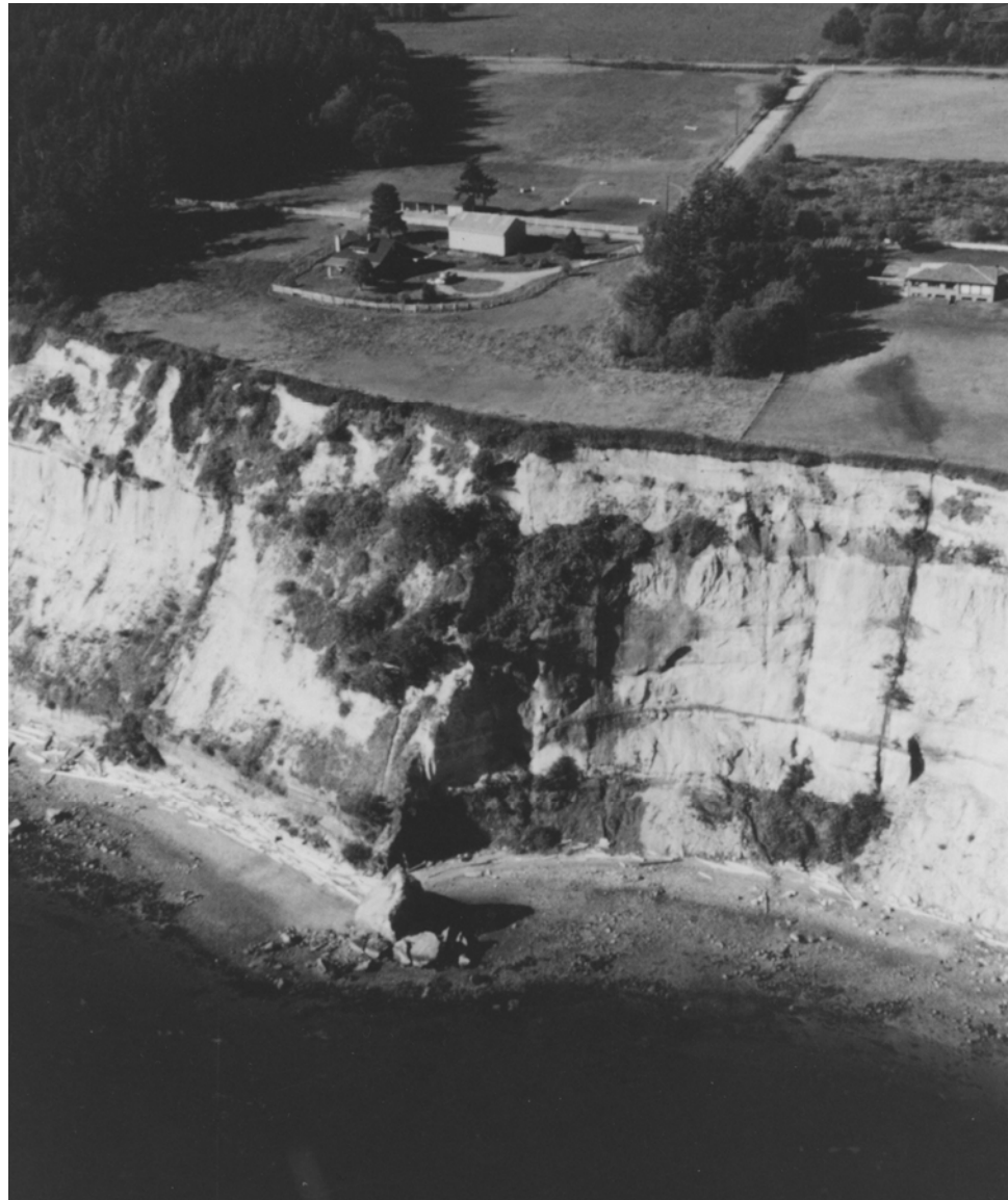
Figure 7. Kloochman Rock, western Oak Harbor, is large enough and close enough to the bluff to slow longshore sediment transport. Longshore drift from the left (south) is reduced, lowering the beach on the right and exposing the bluff there to greater erosion. Erosion rates on either side would not be representative of more distant banks of essentially identical geology and wave action.
