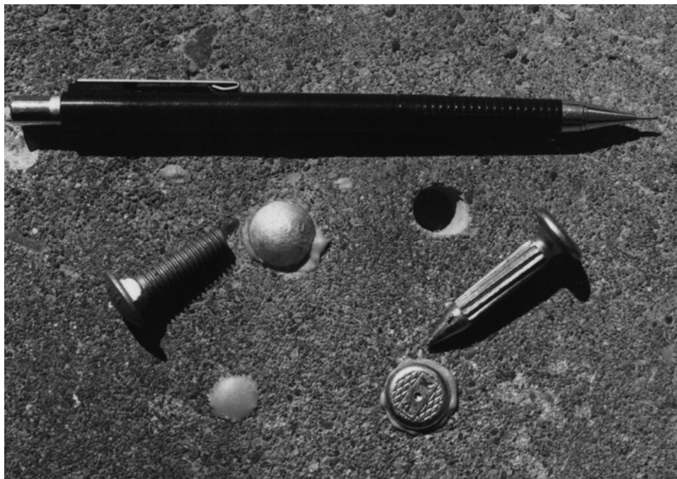
Figure 9. A slab of concrete used to test marking techniques. Gloves and goggles were the only tools that worked “as advertised”. Most glacial boulders are much harder and tougher than concrete. The inset shows a close-up of four holes drilled in a scrap of concrete to demonstrate some options for marking monuments. A common galvanized “carriage bolt” (upper left) is embedded in patching compound. Surveyor s “P.K. nails”, right, can be hammered into asphalt pavement without drilling. A hole (lower left) simply filled with hard-setting compound may be your most durable and vandal-free option.
