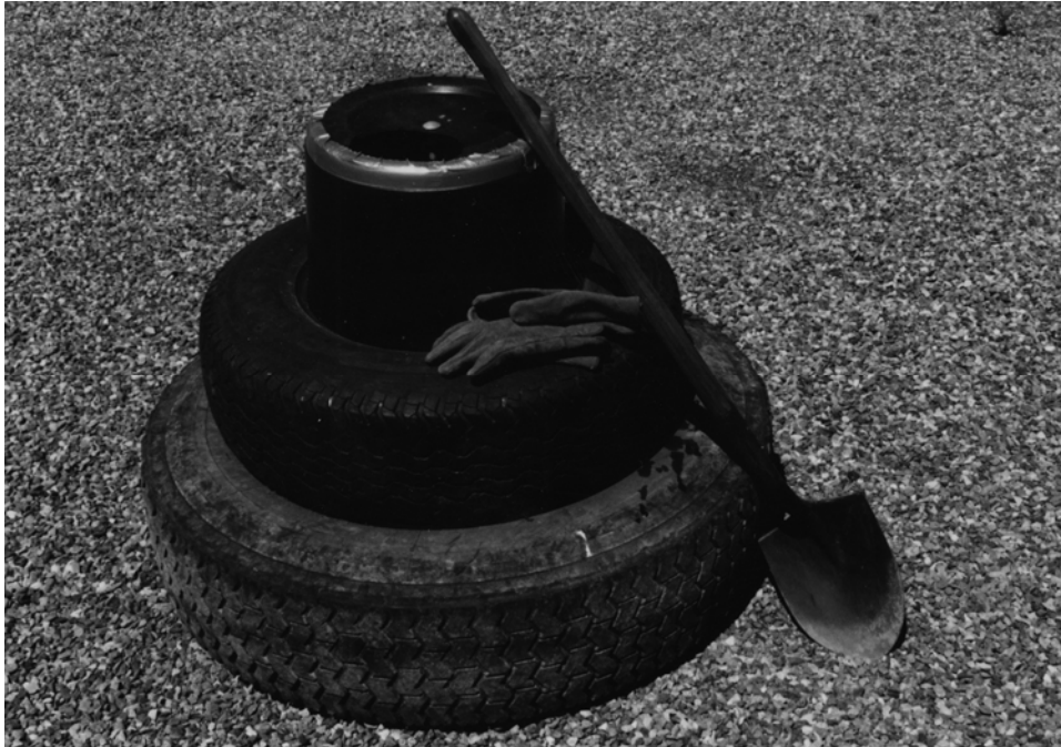
Figure A-2. Concrete monument for monitoring sandy beaches.
