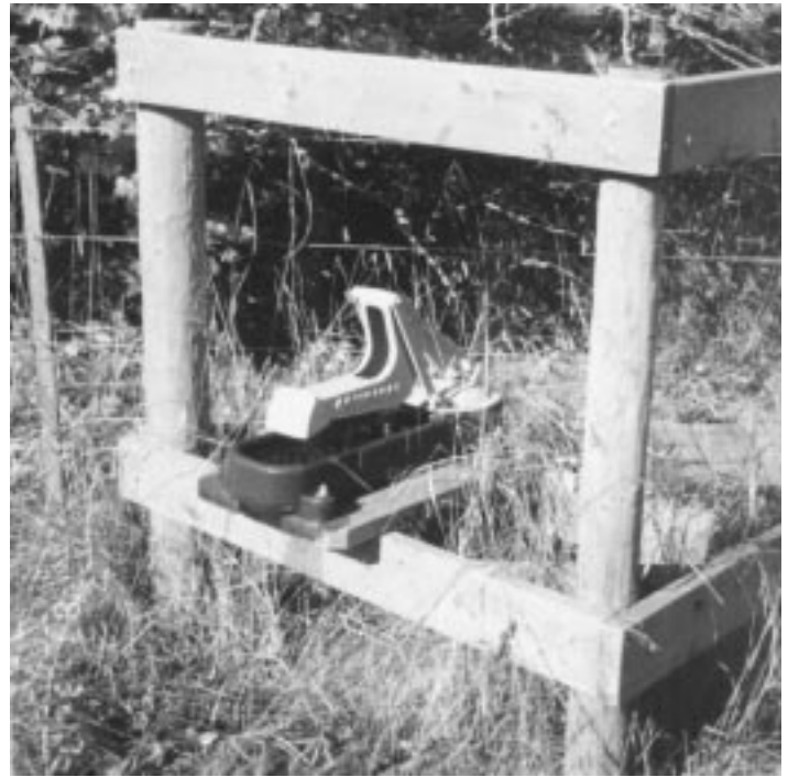
Another alternative for watering the cows is the pasture pump, which takes water from the stream and siphons it up into a small trough. The cow activates the pump by pushing it with its nose.
