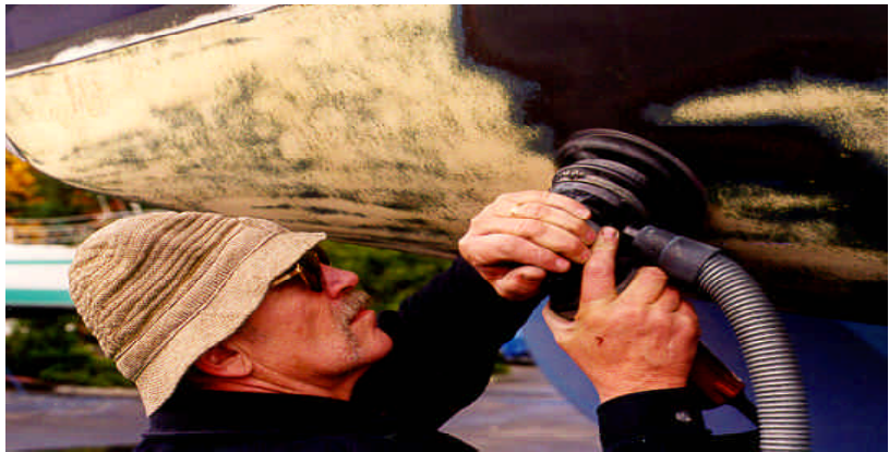
Vacuum sanders clean with 98% of the dust contained in a filter bag, are certified for lead abatement, and workers need only a dust mask and eye protection. Traditional air rotary tools create large volumes of solid wastes, need a respirator and protective coveralls, and the sanding pads gum up rapidly. Photo: Paul Stasch.
