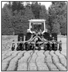
The new "sod injection" from Europe has rapidly caught on in some areas as a way to apply the nutrients in manure to pastures and hay fields. An improvement over overhead spraying, it reduces the potential for water pollution since the liquid waste is distributed evenly into the soil and only goes 4 inches deep. It also reduces odor. The slurry is pumped from the lagoon to the tractor through a hose up to one mile long.
