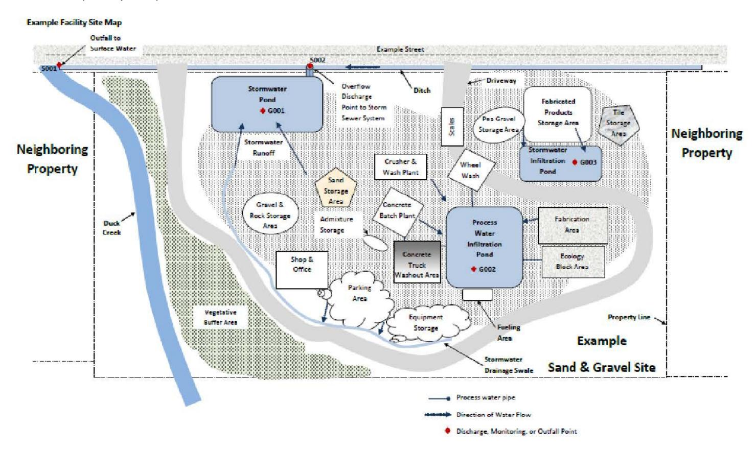
Attachment 3 – Example of how to fill out Sections 14 & 15. Below is a figure that shows example situations of groundwater and surface water discharges from a Sand & Gravel Site. The site below has a NAICS code of 212321. The information from the figure has been used to fill out the section 14 and 15 tables below.
