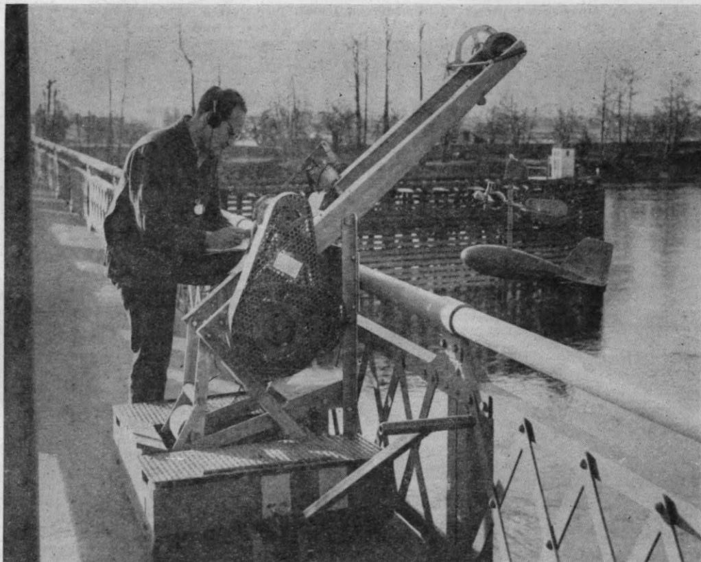
Figure 10. Discharge measurement from highway bridge with battery-power-operated crane. Skagit River near Mount Vernon.
