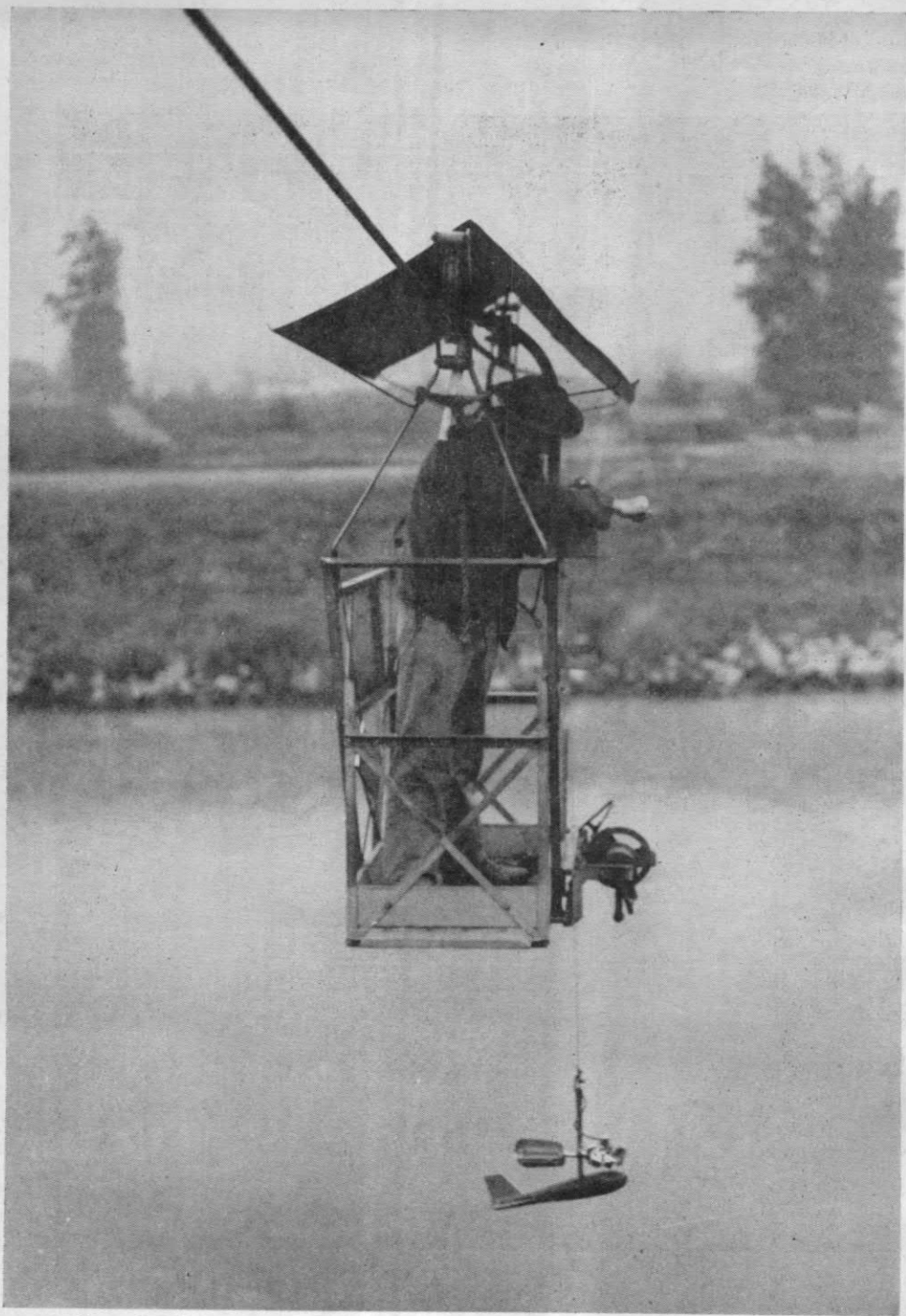
Figure 7. Discharge measurement from standup-type cable car, with current meter suspended above lead weight. Puyallup River at Puyallup.
