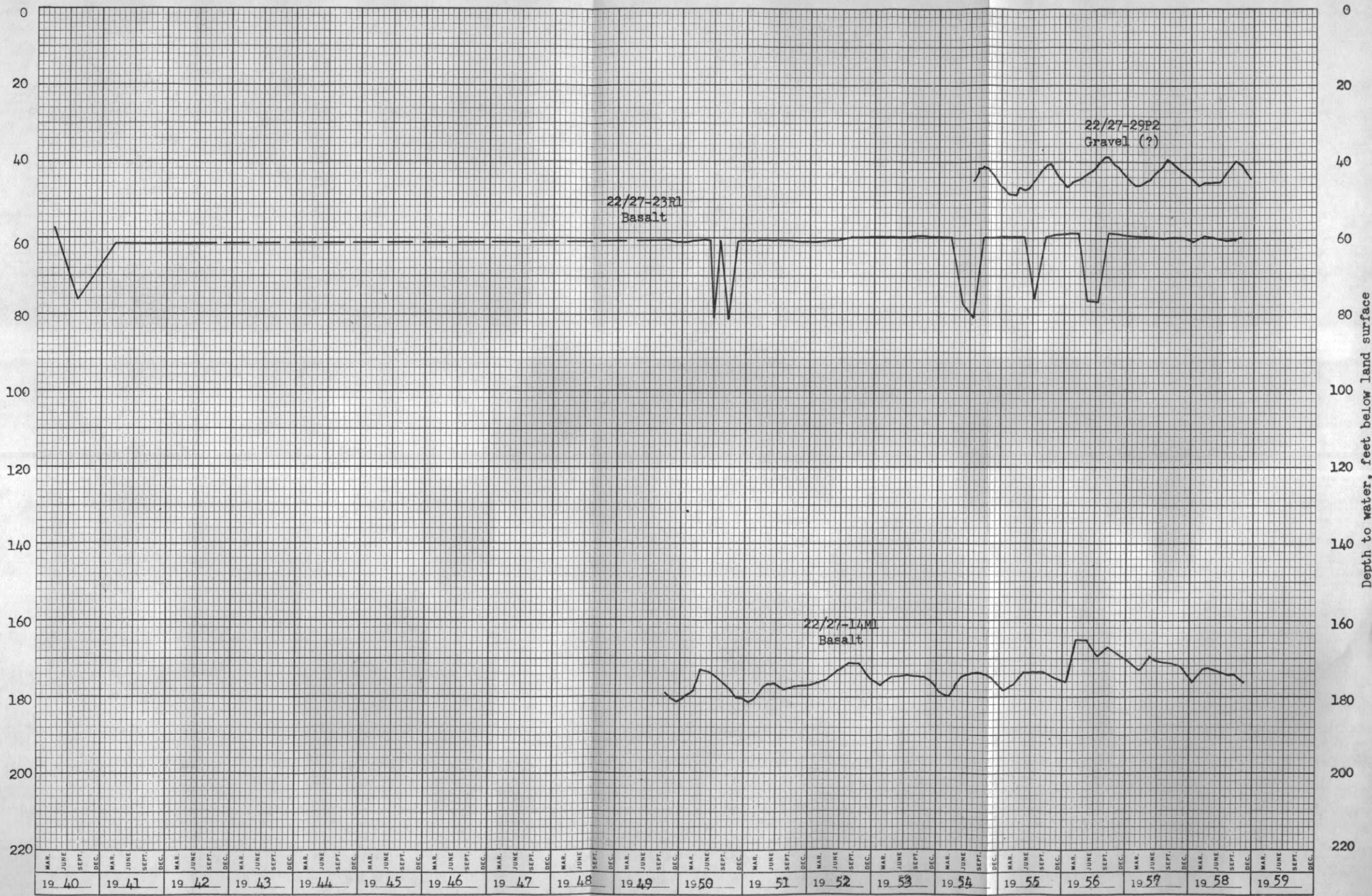
Fig. 23--Hydrographs showing fluctuation of water levels in observation wells.
