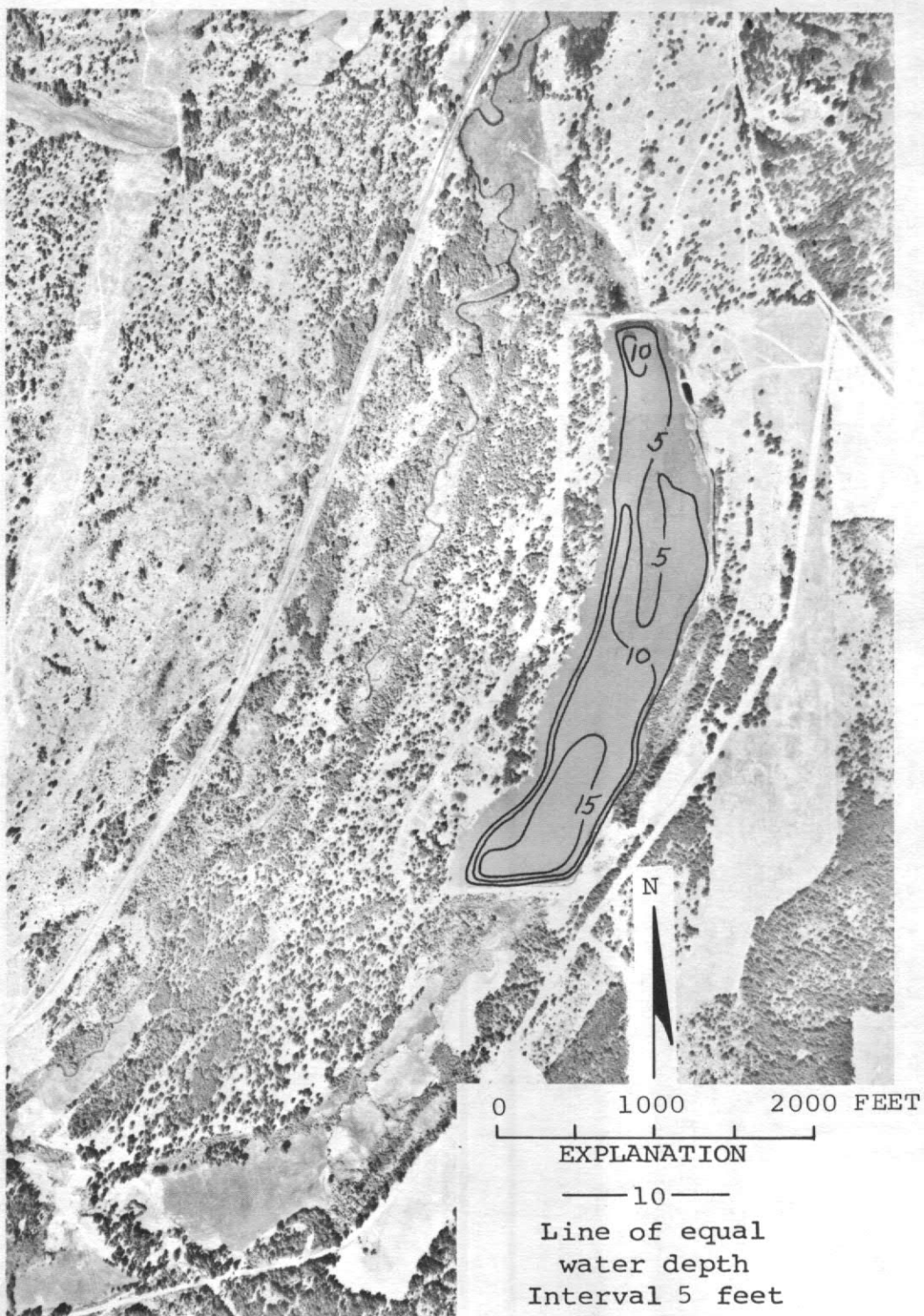
Reflection Lake, Spokane County. Bathymetric map from U.S. Geological Survey, June 11, 1974. Aerial photo, July 2, 1967.
