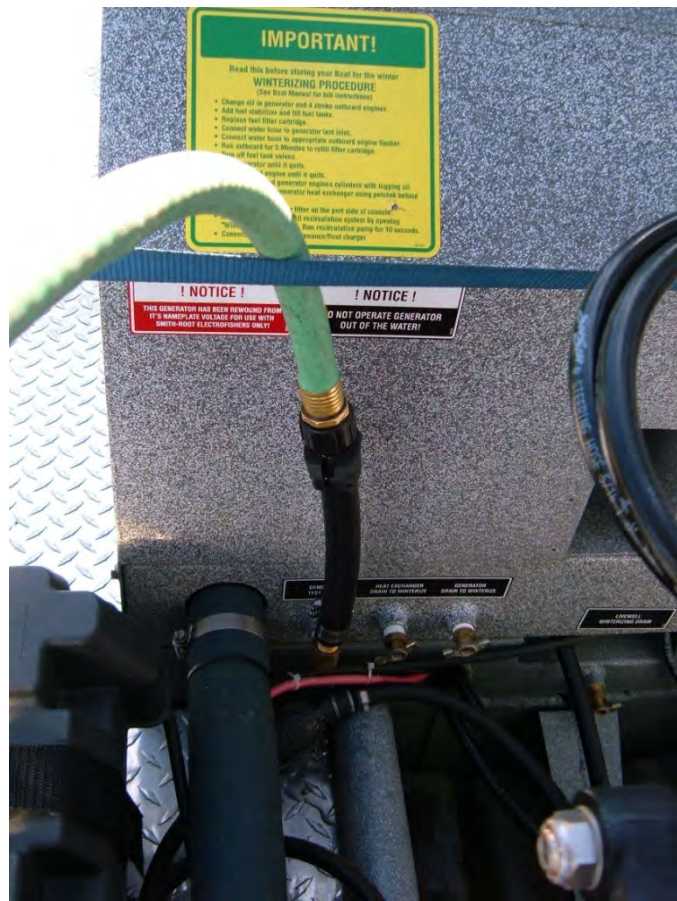
3C. Pipe plug has been removed, and generator flushing adapter has been attached.
