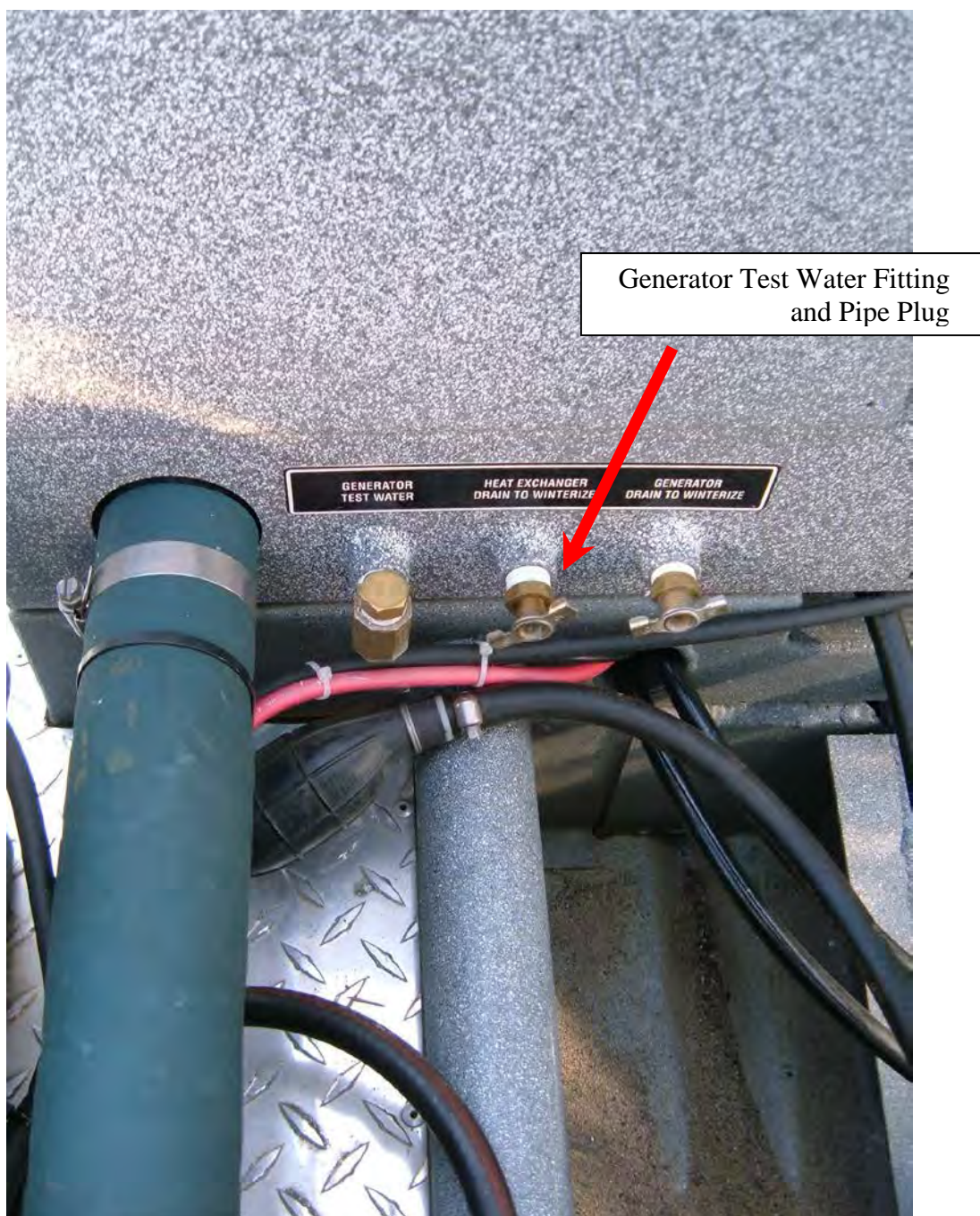
3B. Generator raw water flushing connection (i.e. Generator Test Water Fitting). Located on the base of generator cover, port side aft.
