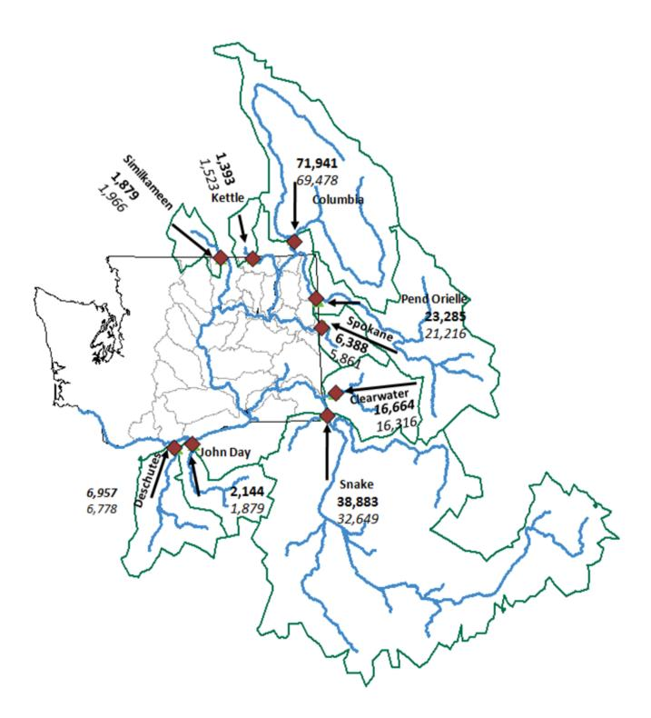
*Figure 7. Surface water flows for major tributaries upstream of the point where the rivers enter Washington state. Top number (bold) refers to 2030 forecasted water supplies for average (50<sup>th</sup> percentile) flow conditions and the middle climate change scenario, while the bottom number (italic) refers to historical (1977-2006) water supplies. All values are in cubic feet per second.*
