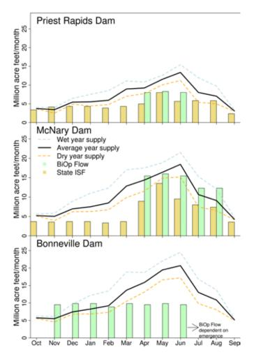
*Figure 15. Historical (1977-2006) surface water supply at Bonneville, McNary, and Priest Rapids dams for low (20th percentile), average, and high (80th percentile) flow conditions. Also shown are the Washington state instream flow (ISF) and federal BiOp flow targets.*
