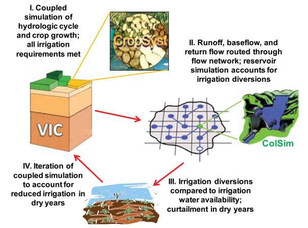
Figure 3. Biophysical modeling framework for forecasting surface water supply and irrigation water demand.
