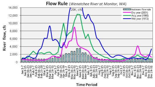
*Figure 11.* Comparison of actual (not modeled) historical flows (1963-2009) during dry (20th percentile), average (50th percentile), and wet (80th percentile) years to the instream flow rule for Wenatchee River at Monitor.
