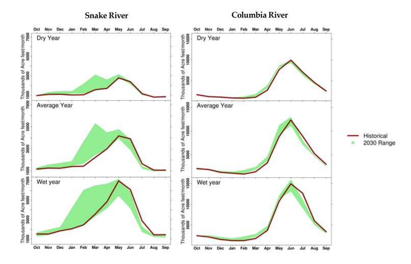
*Figure 8. Historical (1977-2006) and 2030 forecasted regulated surface water supplies on the Snake and Columbia Rivers upstream of the point where they enter Washington state for dry (20<sup>th</sup> percentile, top), average (middle), and wet (80<sup>th</sup> percentile, bottom) flow conditions. The spread of 2030 flow conditions is due to the range of climate change scenarios considered.*
