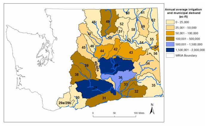
*Figure 14. Total 2030 forecasted average annual surface water and groundwater demands for irrigation and municipal uses (including self-supplied domestic) by WRIA (in ac-ft per year).*
