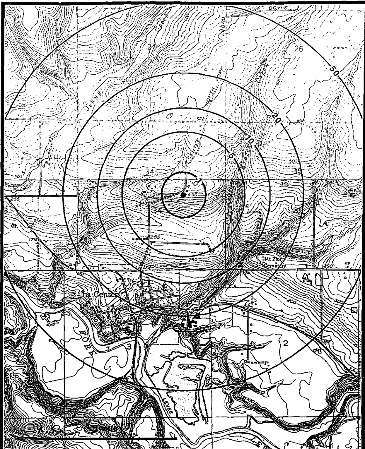
Figure LC-3. 1, 5, 10, 20, and 50 year time of travel zones of contribution using the volumetric flow equation for LaCenter well.
