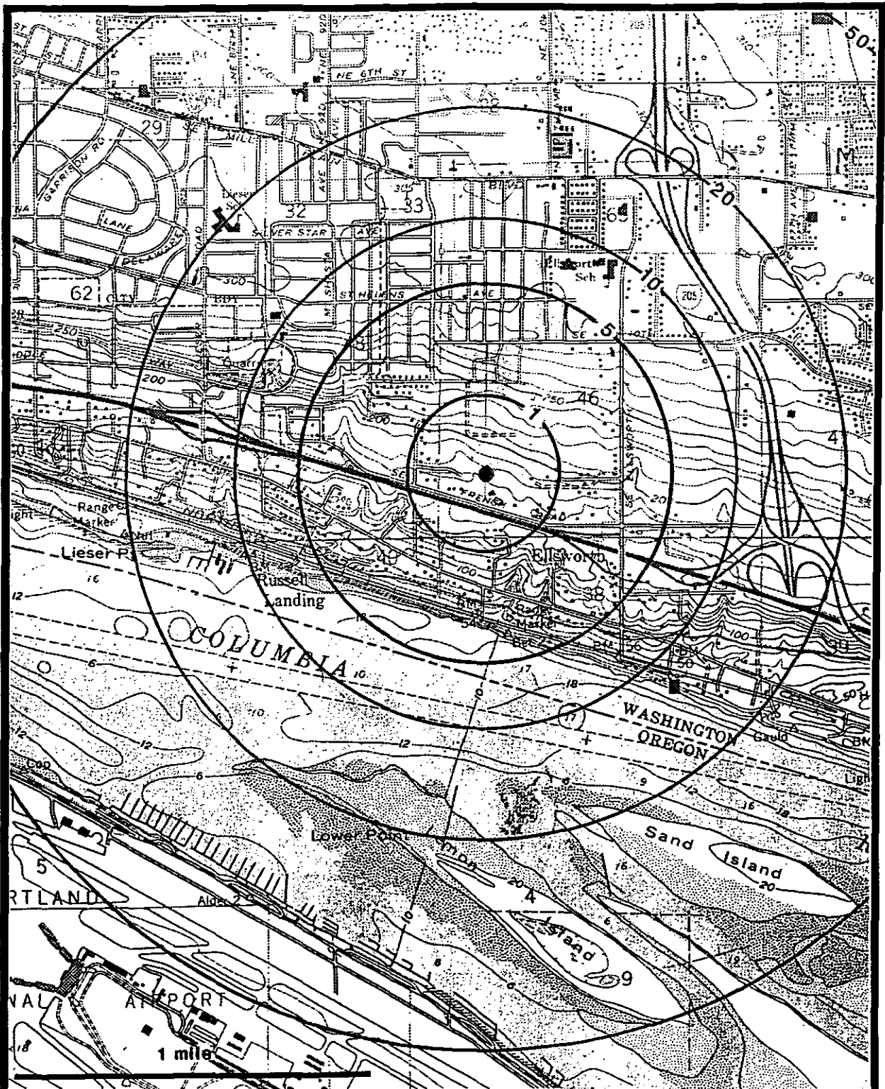
Figure ES-1. 1, 5, 10, 20, and 50 year time of travel zones of contribution using the volumetric flow equation for Ellsworth well.
