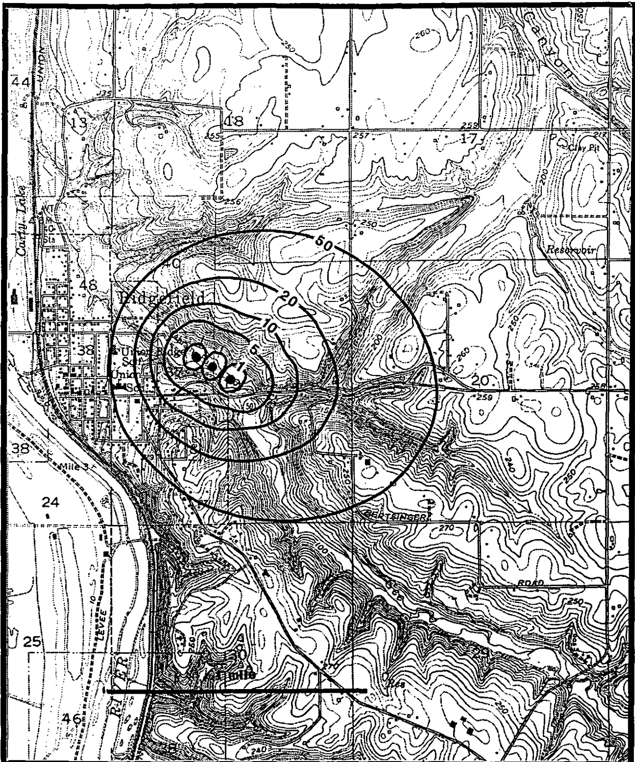
Figure RF-1. 1, 5, 10, 20, and 50 year time of travel zones of contribution for Ridgefield wells 7, 8, and 9 using the EPA RESSQC WHPA model.
