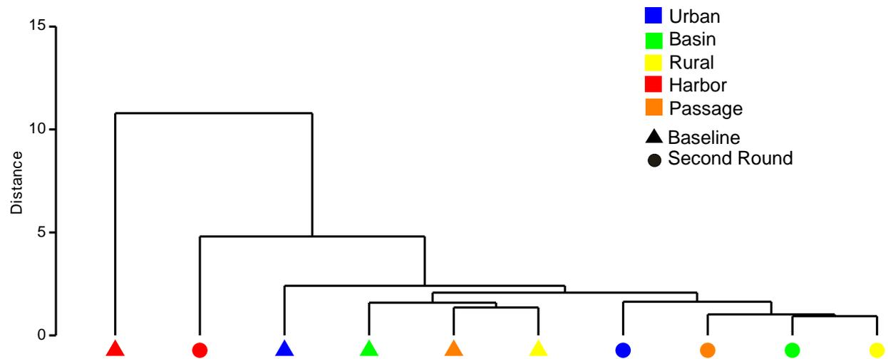
Nonmetric multidimensional scaling (MDS) diagram indicating relative similarities of centroids of stations characterized by 126 chemical parameters for the five sampling strata and two surveys in Puget Sound (unweighted values normalized prior to comparison with Euclidean distance).
