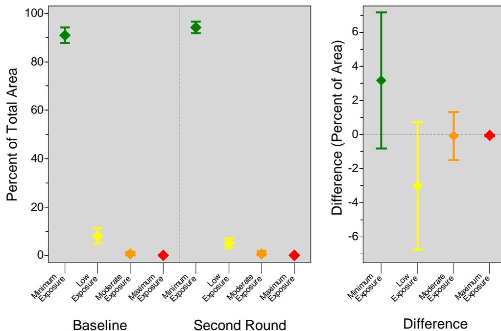
Incidence and spatial extent of chemical contamination, as measured with the Chemistry Index (Dutch et al., 2014), in eight sediment monitoring regions and all of Puget Sound, for each the Baseline (1997-2003) and Second Round (2004-2014) surveys.
