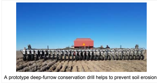
A prototype deep-furrow conservation drill helps to prevent soil erosion.
