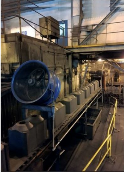
Figure 3: Green (unbaked anodes) on conveyor being transported to the bake ovens.
