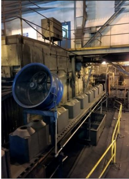
Figure 3: Green (unbaked anodes) on conveyor being transported to the bake ovens.
