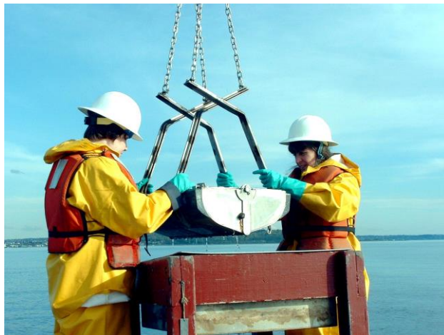
Figure 2. MMU staff landing a van Veen Sampler
