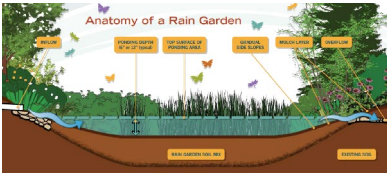
Figure 17: Rain gardens are smaller and less commonly used but have great abilities to infiltrate clean water and keep it clean with the extensive vegetation they are composed of. (WSU Extension).
