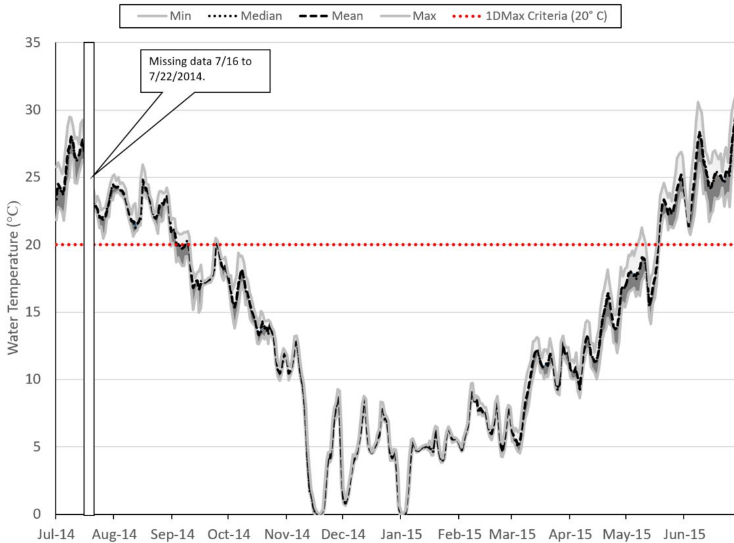
Figure C31: Walla Walla River at Pierce's RV Park (32WAL-09.3) daily summaries of 15-minute temperature data. 1
