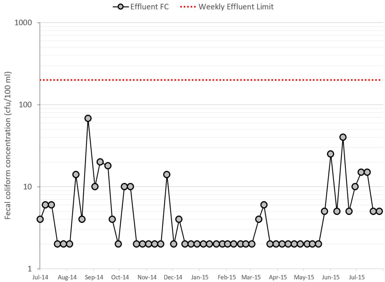
Figure F6: Waitsburg WWTP weekly FC concentrations in effluent discharging to an adjacent wetland on the Touchet River at RM 43.0 versus the weekly NPDES permit limit.
