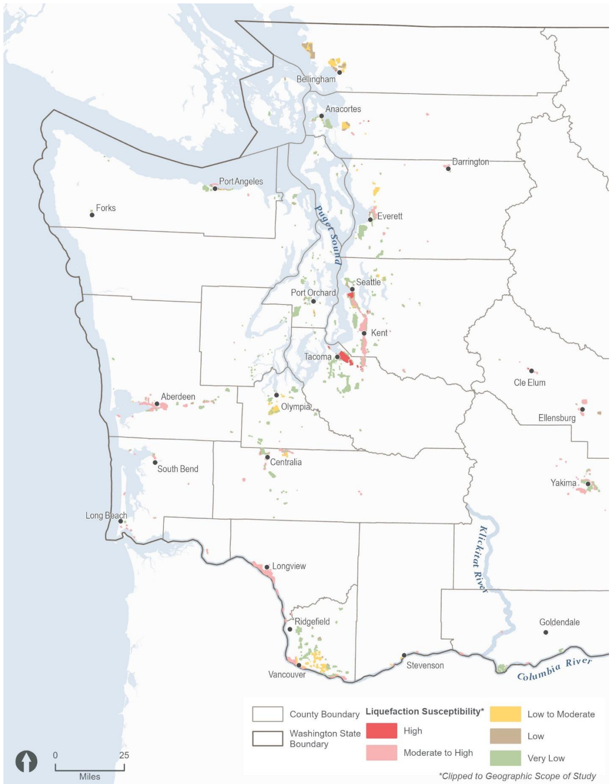
Figure 3. Liquefaction susceptibility in western Washington State
