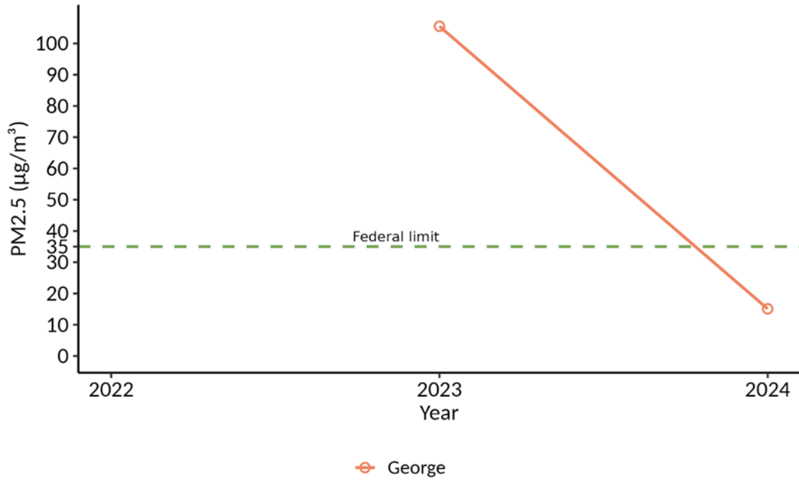
Figure A1. 24-hour PM2.5 (98th percentile) concentrations at the George and West Grant County monitoring site, August 2023-December 2024. Days impacted by wildfire smoke are included. Dashed line is the 24-hr PM2.5 NAAQS (35 µg/m 3 ).
