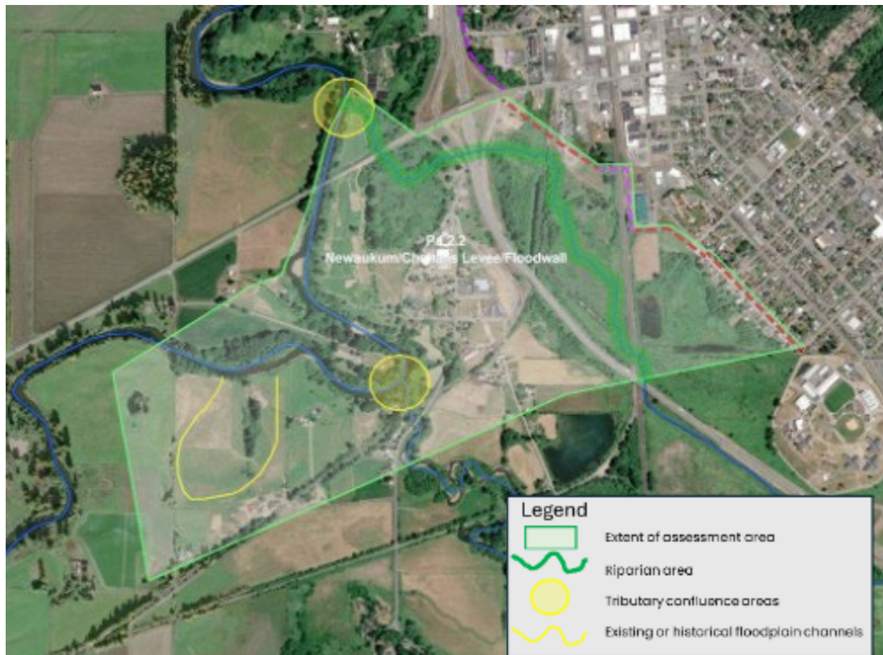
Figure 2: PJ 2.2 East bank of the Newaukum and Chehalis Rivers. Red dashed line is levee; purple dashed line is floodwall. Historical floodplain side channels and riparian corridor offer potential restoration/mitigation opportunities.
