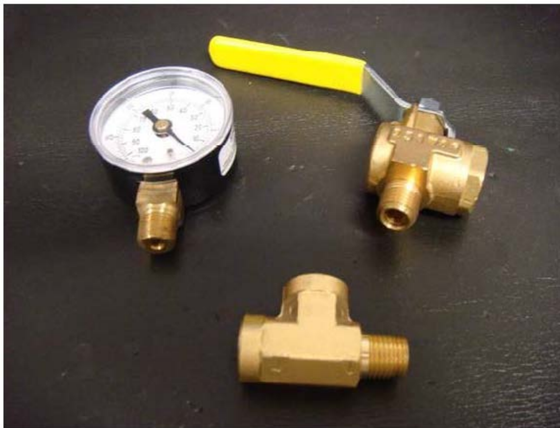
Figure 5-6. Additional hardware needed for full system leak check (Vaughn and Ray, 2011).
