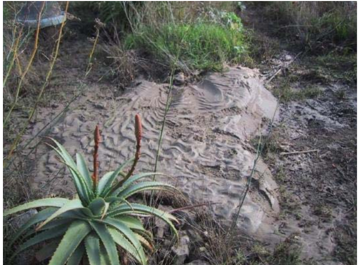
Figure 24: Sand boils resulting from joint failure
