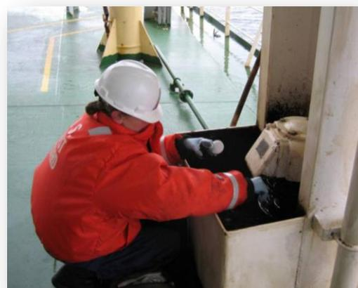
*Figure 5 - A U.S. Coast Guard (USCG) officer takes a sample from the No. 4 starboard fuel oil vent containment box.*
