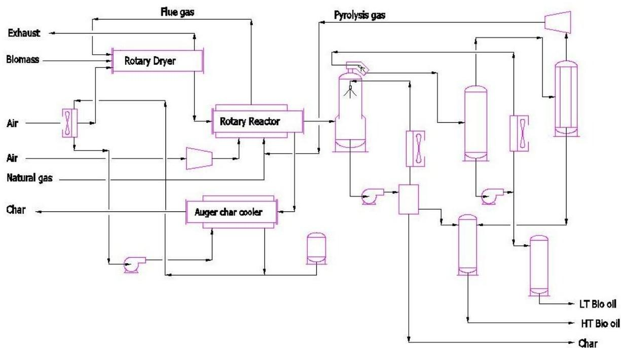
**Figure 9.** Rotary reactor process flow diagram (Courtesy of Coates Engineering, <http://www.coatesengineering.com>).
