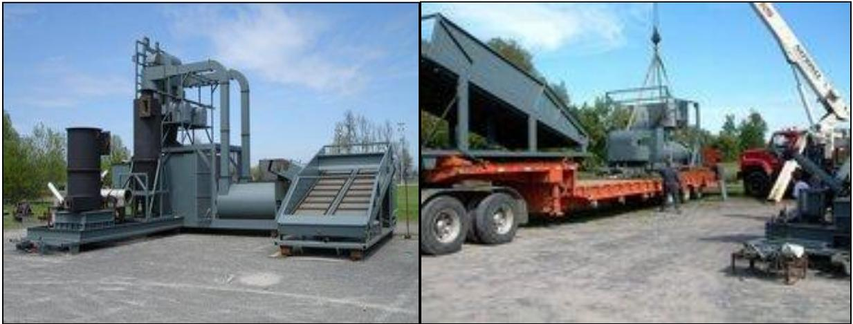
**Figure 22.** This 50 t/day portable (Mobile Pyrolysis Unit, ABRI) must be disassembled for transportation (source: <http://www.advbiorefineryinc.ca/home>; date accessed: Nov., 15, 2010).
