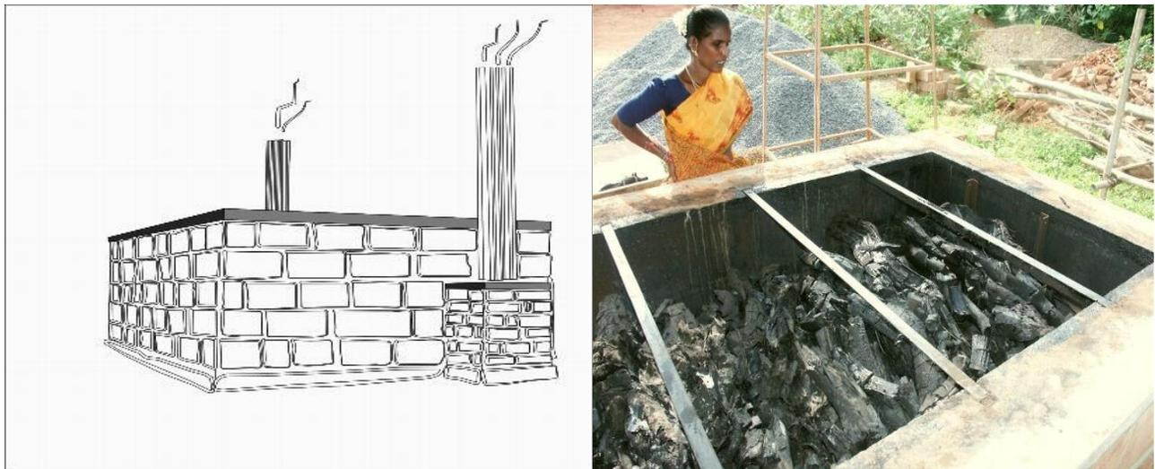
**Figure 43.** Improved Charcoal Production Systems (ICPS) or Adam retort (source: <http://www.biocoal.org/3.html>, date accessed: Nov. 15, 2010).
