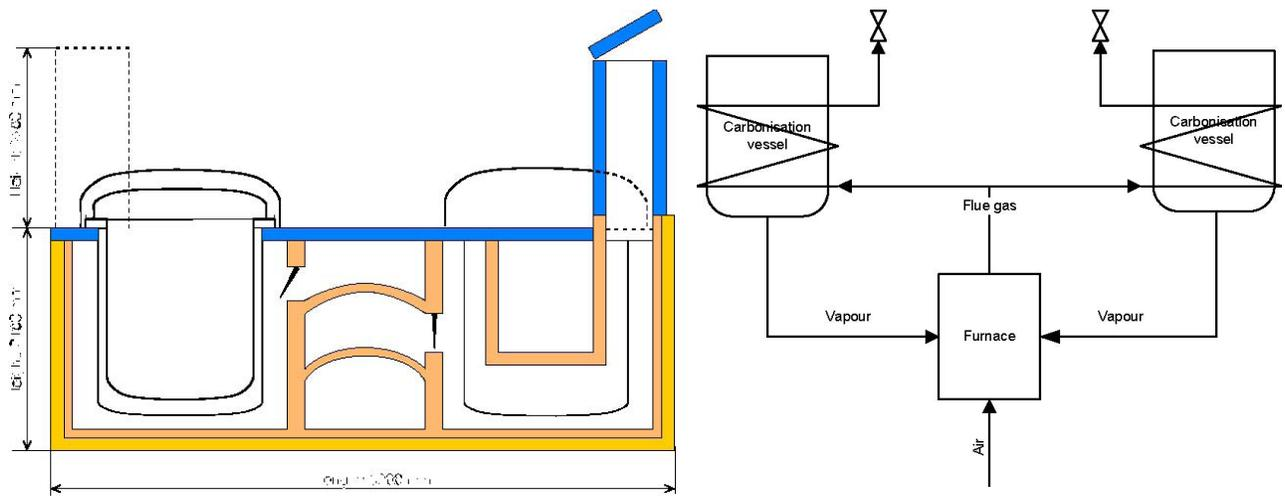
**Figure 15.** Cross section of the Carbo Twin Retort and operating principles (Trossero et al., 2008).
