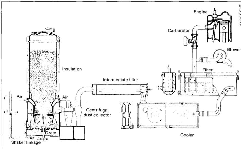
**Figure 82.** Producer gas engine for spark ignition system (SERI, 1988).
