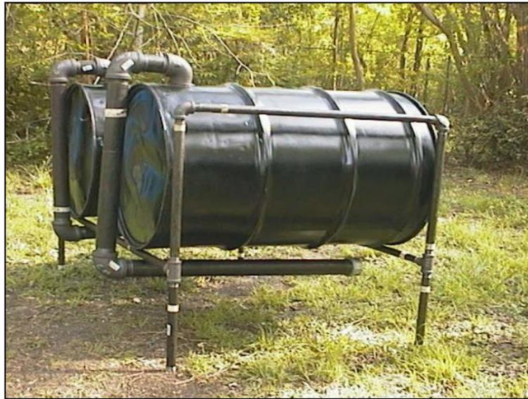
**Figure 47.** Small retort constructed of oil drums ([http://www.twinoaksforge.com/BLADSMITHING/MAKING% 20CHARCOAL.htm](http://www.twinoaksforge.com/BLADSMITHING/MAKING%20CHARCOAL.htm), date accessed: Nov. 13, 2010).
