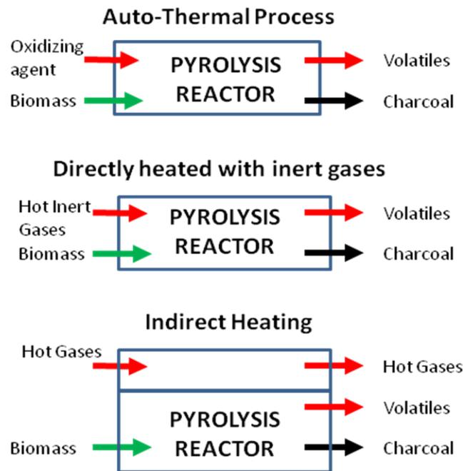
**Figure 18.** Types of pyrolysis technologies according to the heating method used (Fournier, 2009).
