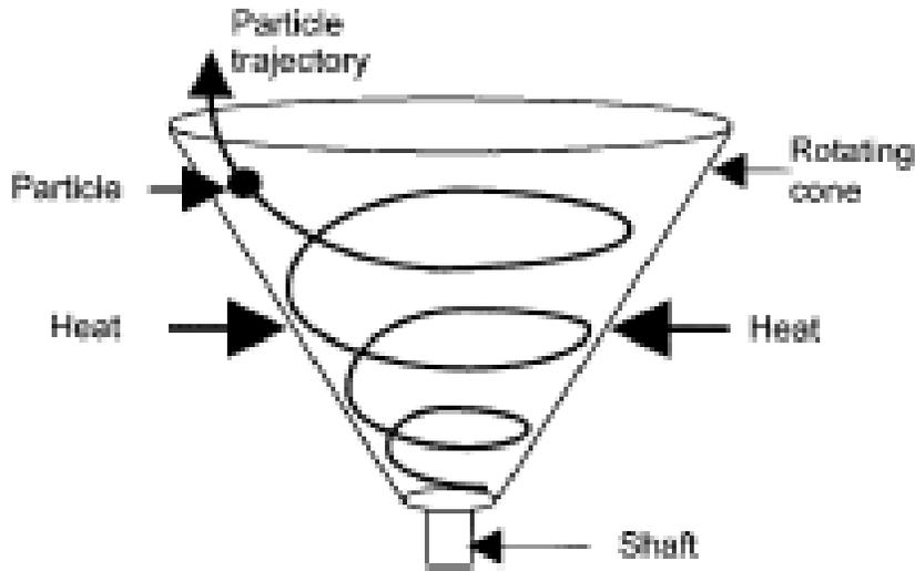
**Figure 79.** University of Twente rotating cone principle (Bridgwater and Peacocke, 2000).
