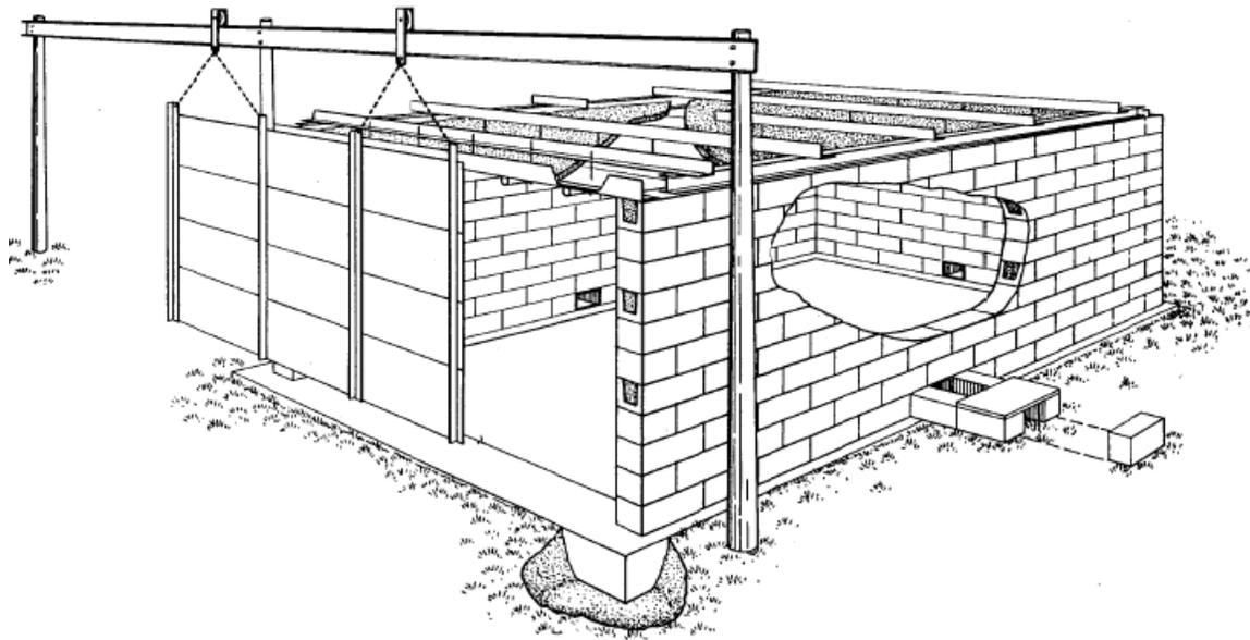
**Figure 42.** A single wall masonry block kiln of seven cord capacity (cinder block biochar kiln) (Toole et al., 1961).
