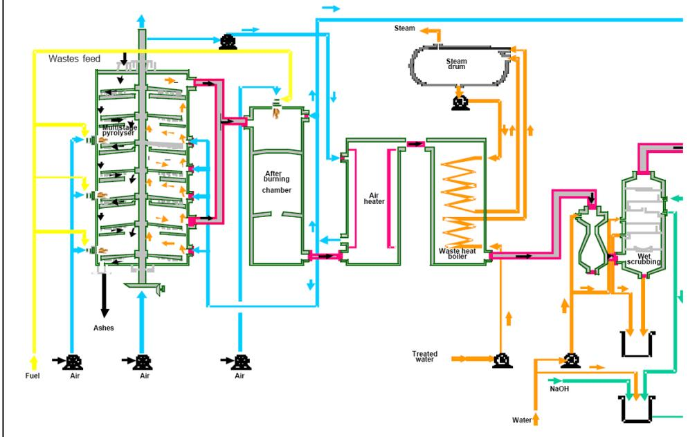
Figure 61. NES A stationary multiple hearth kiln (<http://www.cmigroupe.com/nesa/pdf/Pyrolysisof.pdf>, date accessed February 2010).
