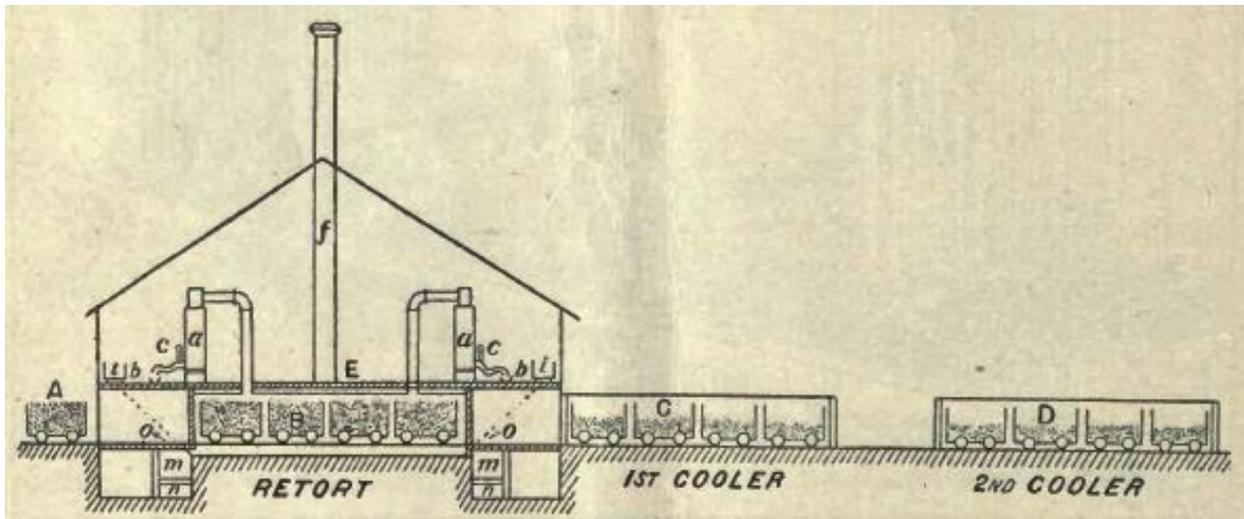
**Figure 49.** Plan of a American destructive distillation plant in continuous operation. A: car, B: retort, C: first cooler, D: second cooler, E: acetate drying floor (Veitch, 1907).
