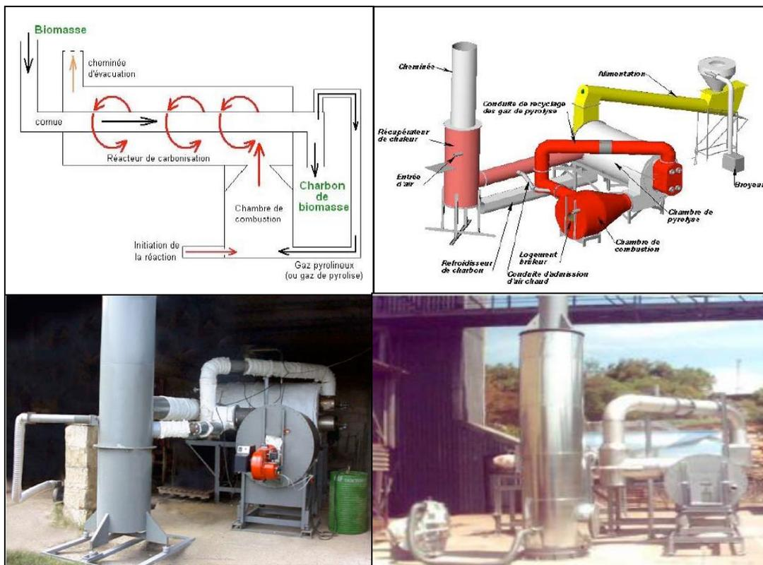
**Figure 31.** Continuous reactor indirectly heated through the walls with the heat released from the combustion of pyrolysis vapors (source: <http://www.pronatura.org/index.php>) (date accessed: Nov., 15, 2010).
