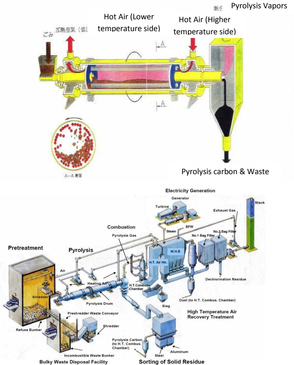
**Figure 62.** Pyrolysis rotary drum, Mitsui Recycling ([http://www.ieabcc.nl/meetings/Tokyo\\_Joint\\_Meeting\\_/02Mitsui.pdf](http://www.ieabcc.nl/meetings/Tokyo_Joint_Meeting_/02Mitsui.pdf), date accessed: Nov. 13, 2010).
