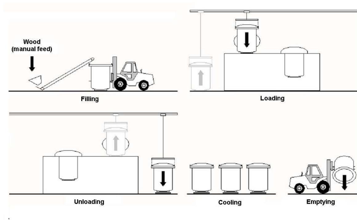
**Figure 16.** Operating principles of a semi-batch system (Carbo-Twin Retort) (Trossero et al 2008).
