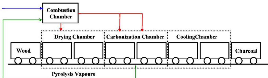
**Figure 17.** Continuous carbonization operations use pyrolytic vapors to heat the combustion chamber (Trossero et al., 2008).
