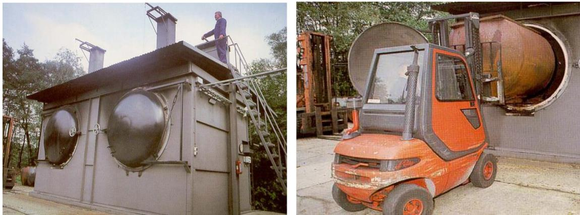
**Figure 14.** Semi-batch reactor - Van Marion Retort (VMR) system (source: <http://www.bioforsk.no/ikbViewer/Content/71499/Biokarbonseminar%20%C5s%2011-03-2010%20Morten%20Gr%F8nli.pdf>) (date accessed: Nov., 14, 2010).
