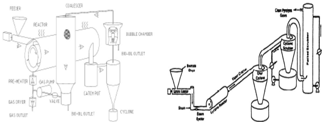
**Figure 76.** Ablative fast pyrolysis reactors (Graham et al., 1984).
