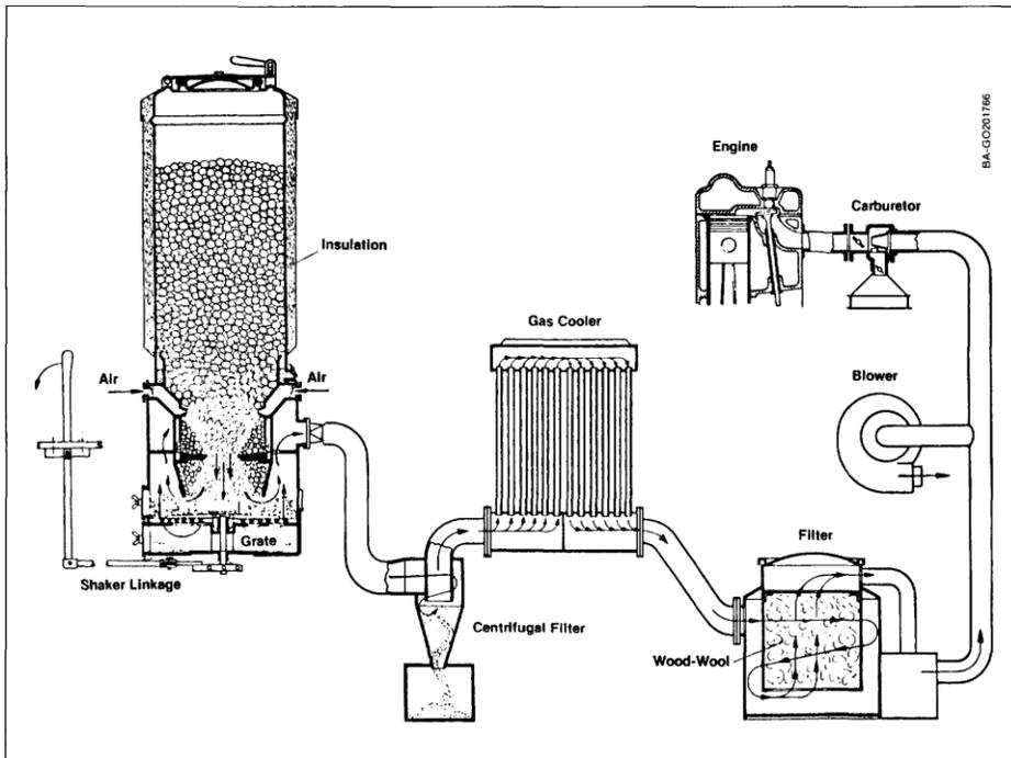
**Figure 81.** Typical vehicle gasifier showing cyclone and gas cooler (SERI, 1988).
