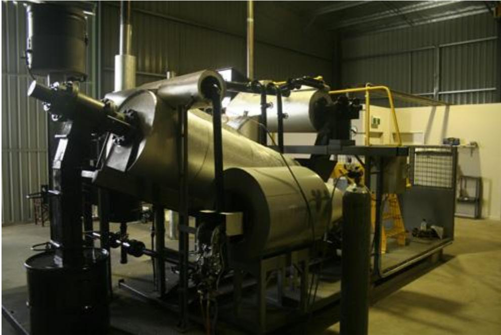
**Figure 69.** eGenesis CR-2 pyrolysis unit for the production of biochar and synthesis gases (<http://www.egenindustries.com/>, date accessed: Nov. 13, 2010).
