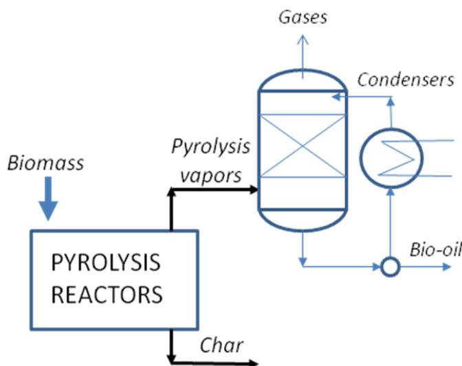
**Figure 8.** Pyrolysis scheme for the production of biochar, bio-oil, and gases (Pelaez-Samaniego et al., 2008).
