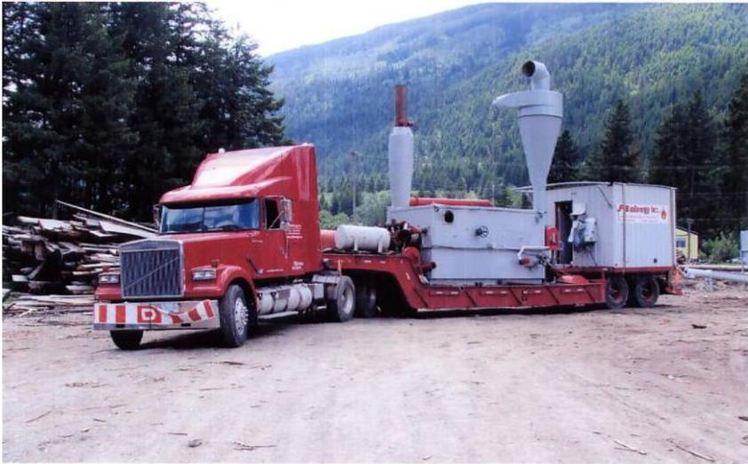
**Figure 23.** Mobile pyrolysis reactor developed by JF Biocarbon, Canada (source: <http://terrapreta.bioenergylists.org/taxonomy/term/1175>; date accessed: Nov., 15, 2010).
