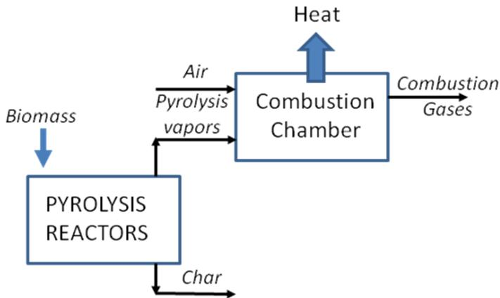
**Figure 4.** Pyrolysis scheme for the production of biochar and heat (Pelaez-Samaniego et al 2008)
