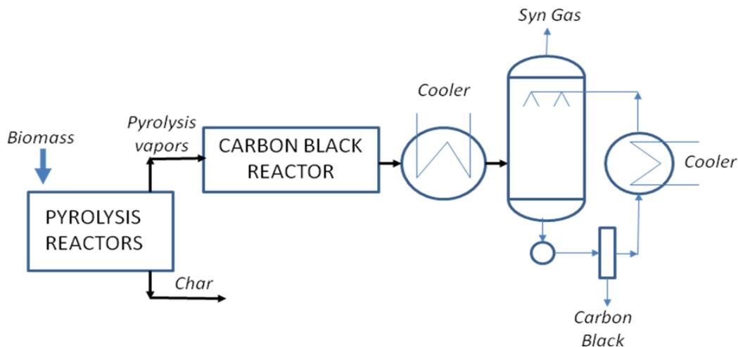
**Figure 11.** Pyrolysis process for the production of biochar, carbon black, and syngas (Pyrolysis reactor temperature 400-550 °C, carbon black reactor temperature over 1200 °C) (Pelaez-Samaniego et al., 2008).
