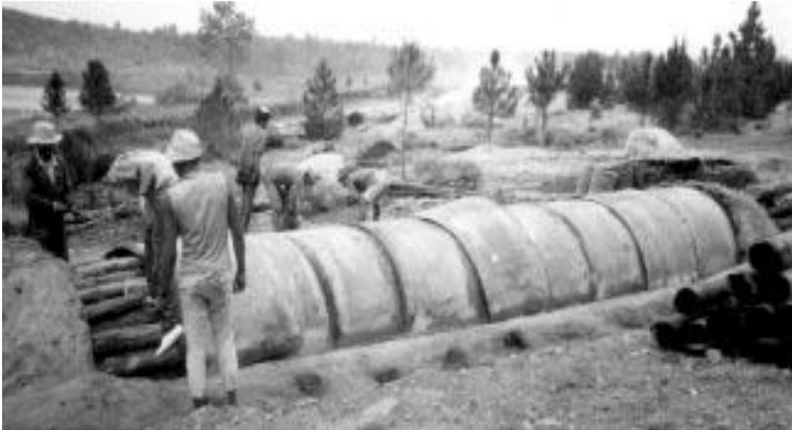
**Figure 37.** Improved earth kiln design. A semi-permanent, low-cost, earth-metal kiln in Madagascar (Girard, 2002).
