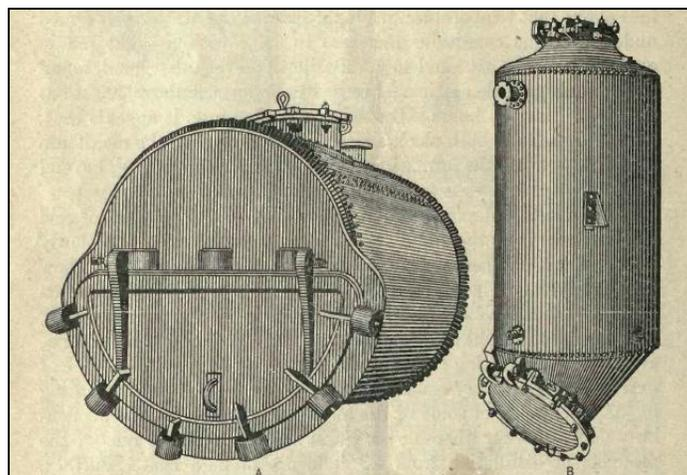
**Figure 26.** Horizontal and vertical retorts used in distilling turpentine (Veitch, 1907).
