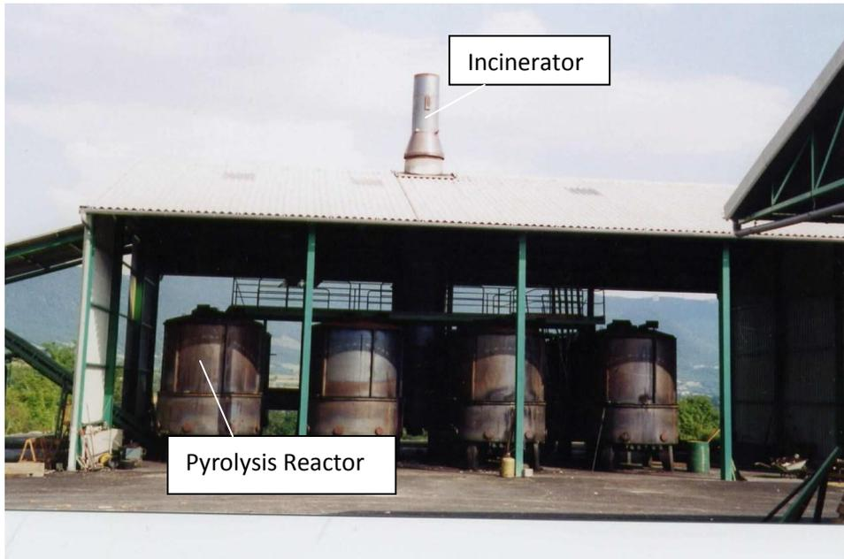
**Figure 6.** CML process for heat recovery in batch systems (CIRAD and Innov-energies, 2007).
