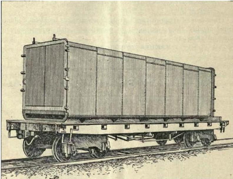
**Figure 51.** Biochar cooler used with oven retort (Veitch, 1907).
