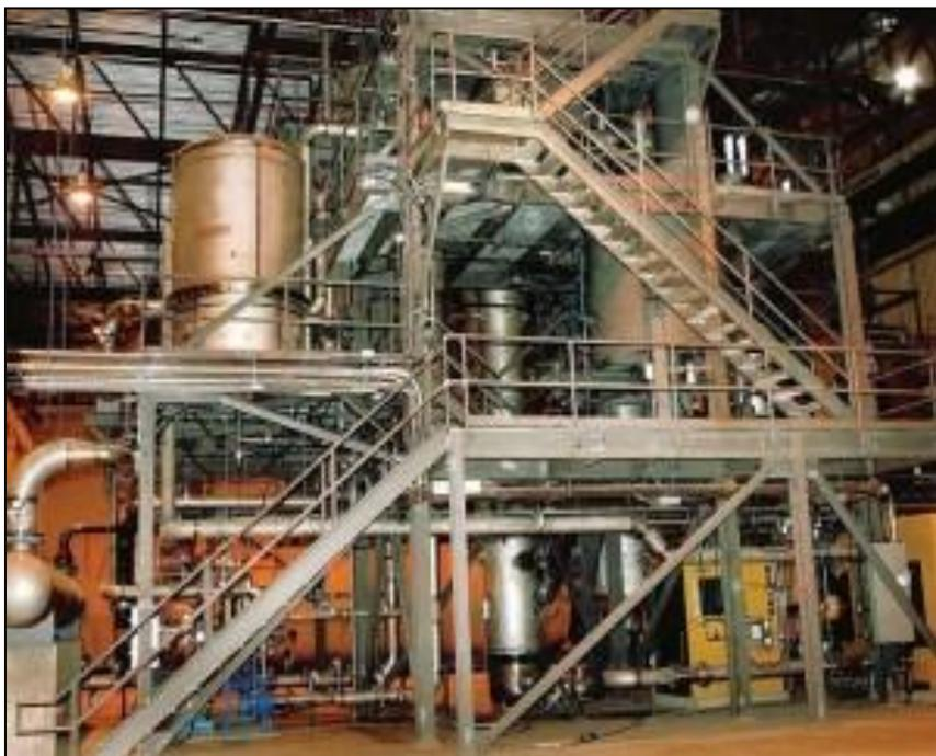
**Figure 75.** Circulating bed pyrolysis reactor (<http://www.uop.com/renewables/10060.html>, date accessed: Nov. 13, 2010).
