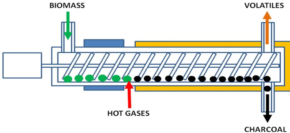
**Figure 64.** Auger reactor.
