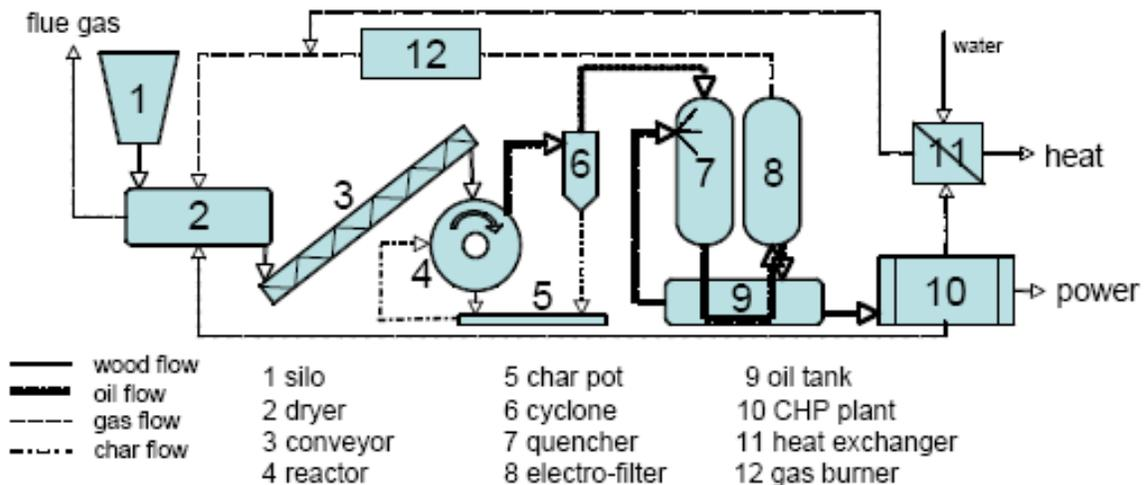
**Figure 77.** Pytec's biomass to oil ablative pyrolyser from the University of Hamburg (Venderbosch and Prins 2009).
