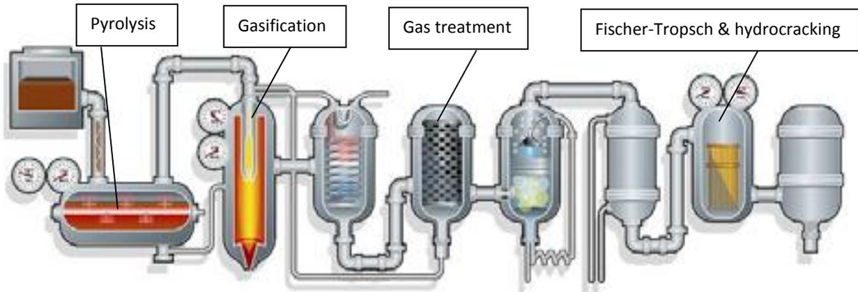
**Figure 13.** The Choren process for producing syngas using paddle pyrolysis reactors (Bienert, 2007).
