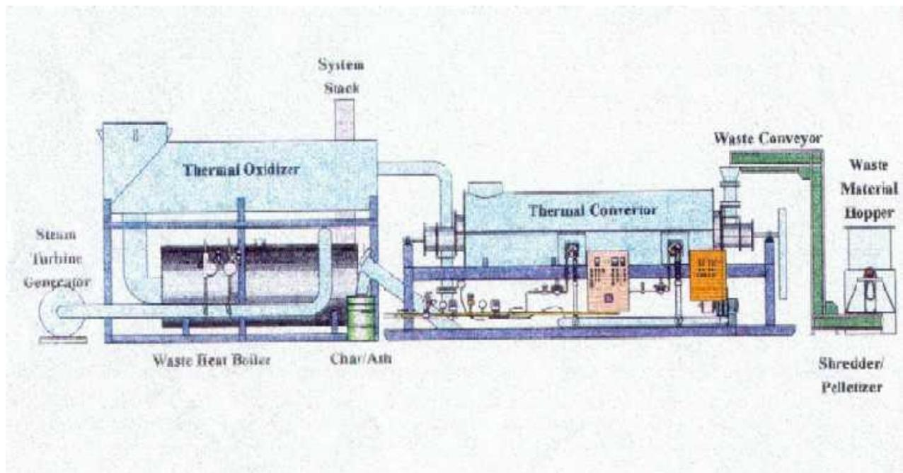
**Figure 5.** Pyrolysis unit with heat recovery (International Tech Corporation)
