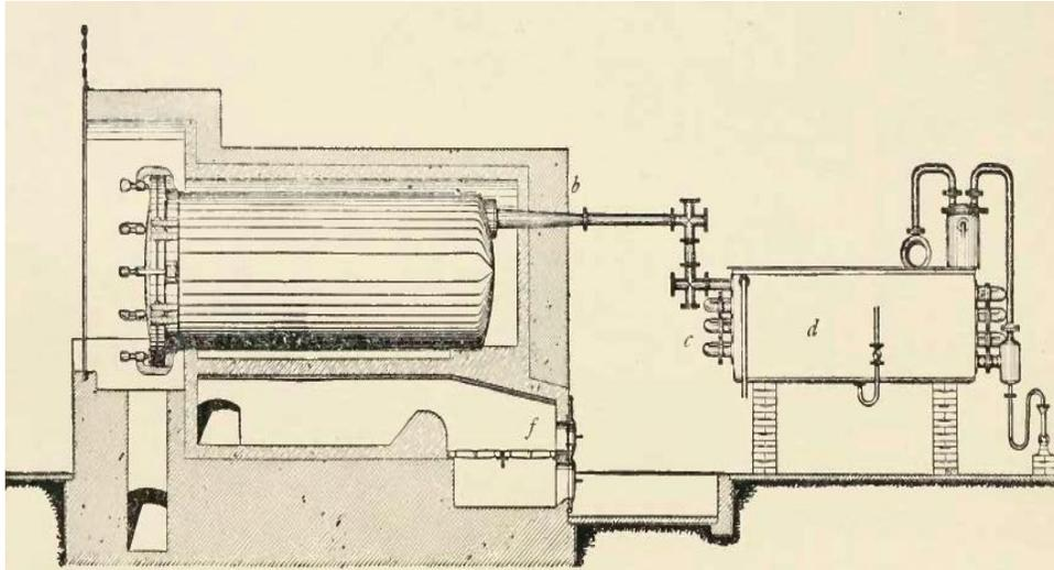
**Figure 48.** Horizontal steel retort (capacity 1.5 stacked m<sup>3</sup>, operating period 12-16 hours a-retort, b-retort neck, condenser tubes, d-condenser tank, f- furnace) (Klark, 1925).
