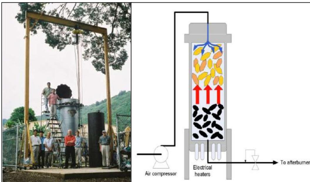
**Figure 32.** High-pressure pyrolysis reactor at the University of Hawaii (Antal, 2009) ([www.hnei.hawaii.edu](http://www.hnei.hawaii.edu); date accessed: Nov. 13, 2010).
