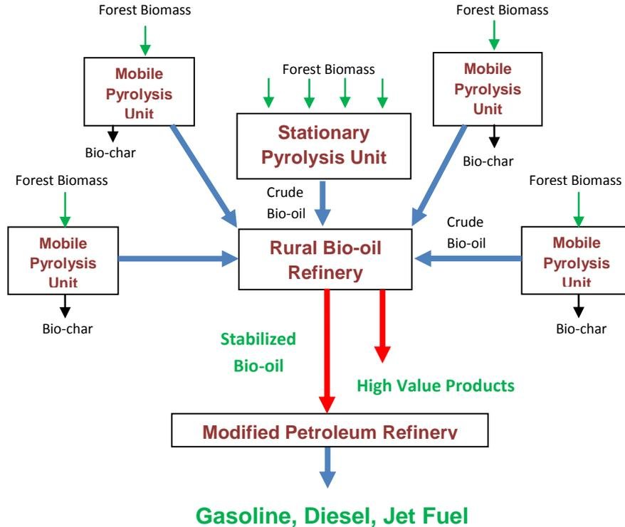
**Figure 10.** Biomass economy formed by mobile and stationary pyrolysis units, by rural refineries and by a modified petroleum refinery.
