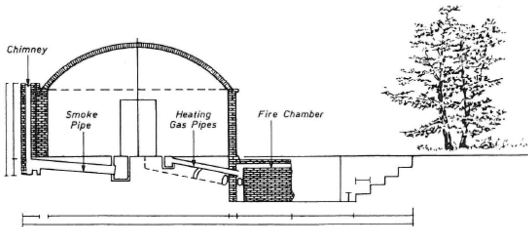
**Figure 38.** The Beehive fire brick kiln with external heating (Emrich, 1985).
