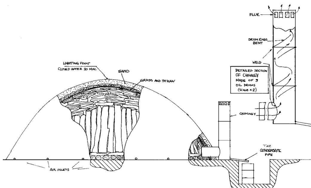
**Figure 35.** An earth-mound kiln with pyrolysis oil recovery (FAO, 1987). *Image courtesy of the Food and Agriculture Organization of the United Nations.*
